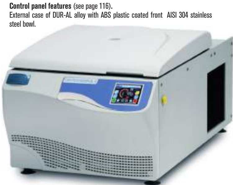
Model “Centrofriger BLT” refrigerated, temperature range -12 °C to 40 °C.
