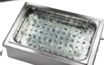
Stirring detail by internal circulation pump.
