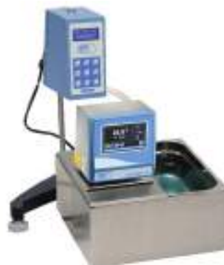
Immersion thermostat Digiterm controlling temperature of viscometer.
