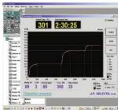
The software included makes easier the digestion program edition and the digester temperature register.
