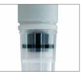
Visual inspection! A resilient sealing ring not only adapts the pipette to small tip variations, but also provides a very distinct visual check for the correct seating and sealing of the tip.
