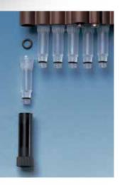
Individual shafts with seals can be easily unscrewed with only a simple gripping tool, which is supplied. Tip cones and seals can now be easily cleaned or replaced. This patented procedure eliminates the expense and long downtime associated with sending pipettes out for service, ensuring long service life and low operating costs. Recalibration is not required!
